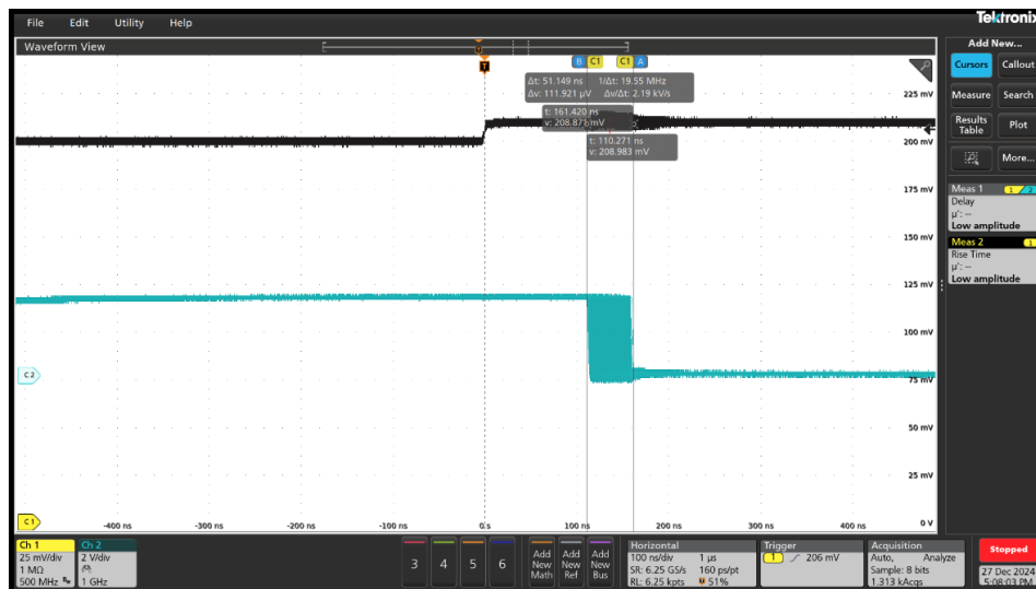
CH1: IN 25mV/div, CH2: OUT 2V/div, 示波器余晖模式
